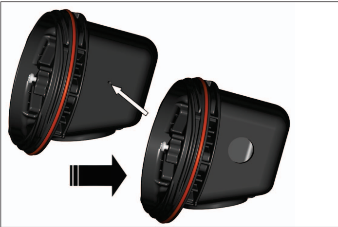
14. Using dimple molded into side of junction box base to locate center of hole, drill for supplied connection fittings per manufacturer's recommendation.
