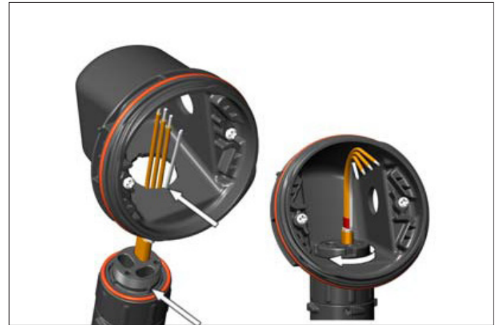
15. Mount junction box base on expediter. Make sure to align slot to properly orient junction box base.
