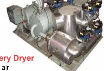
Dual Tower D<sub>2</sub>O Vapour Recovery Dryer
