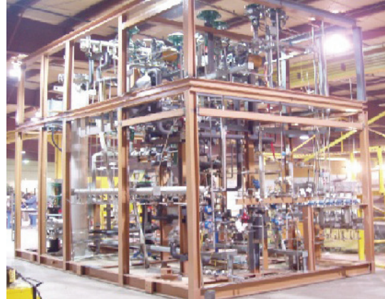
Engineered Module Tritium Removal Facility Dryer Skid
