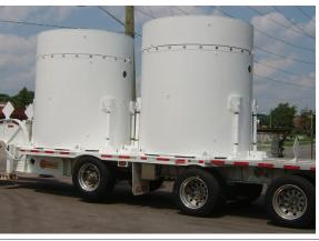
The Multi Purpose Transportation Package is designed to safely transport radioactive material from a nuclear plant to the disposal site. The unit is designed to withstand a severe fall and mounts on a special trailer.
