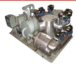
The Twin Tower Dryer works the same way as a Single Tower Dryer, except that it provides continuous operation because one tower is regenerating while the other is adsorbing.
