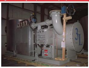
The Single Tower D<sub>2</sub>O Vapor Recovery Dryer removes heavy water vapor from reactor buildings. It consists of a tower filled with desiccant. Wet air is forced into the desiccant tower which absorbs water moisture. Dry air is re-circulated into the building. Desiccant is regenerated by passing hot air through it. Moisture is picked up by the hot air and condensed to recover heavy water.
