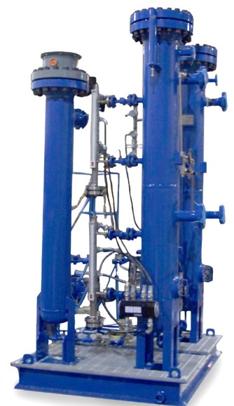
3 Stages – Duplex Separation, pressure reducing, and dew point control. Gas electric heating technology.
