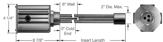
Figure 39 - 2" NPT Screwplug (Three Straight Elements)
