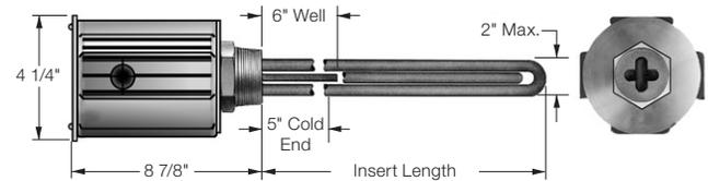
Figure 38 - 2" NPT Screwplug - Two Hairpin Elements
