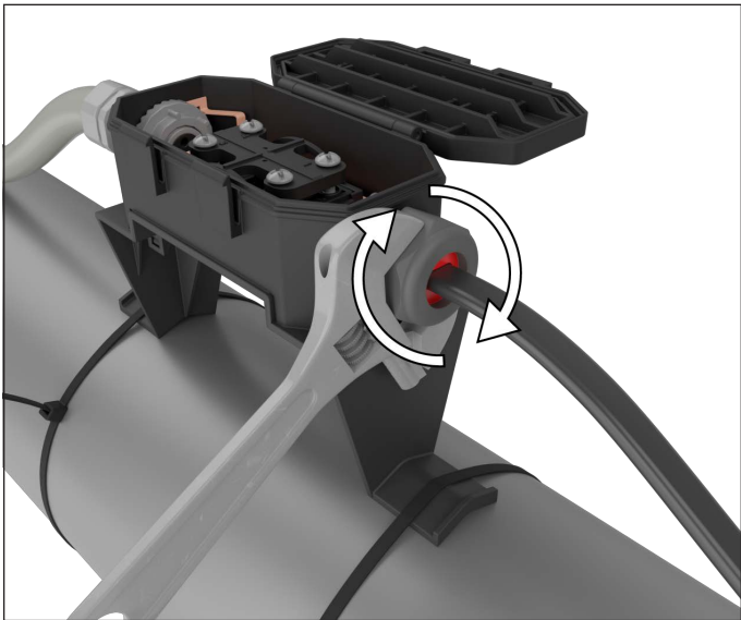
8. Torque gland nut (8 Nm for "LINK-B" version, 5 Nm for "LINK-D" version) to seal around cable.
