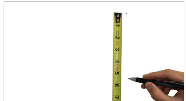
Figure 9 – Measure and scribe the top and bottom hole locations and drill holes
