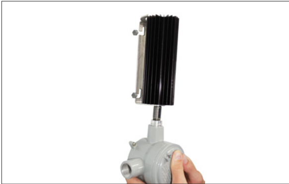
Figure 10 – Position heater onto mounting bolts
