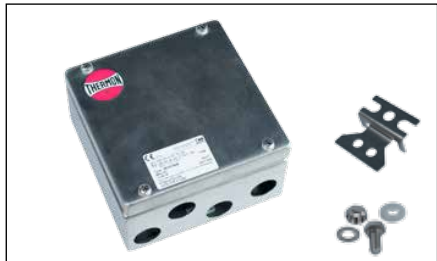
JB-SS-150. Thermon's Junction Box SS is a wall mounted, tracer/power box, 316 stainless steel. 4 x 25mm Entries, Terminal block c/w two jumpered pairs, L1 and L2 and two Earth terminals, Enclosure rating is IP66. External dim.150mm x 150mm x 81mm, IECEx Approval EMC-SS... External Mounting Clips to suit JB-SS-150 (ordered Separately)
