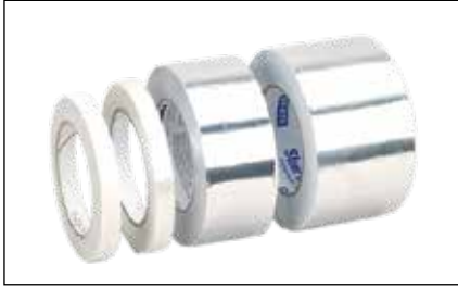
FT-1H... fixing tape for attaching heating cable to piping every 300 mm or as required by code or specification.
