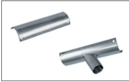
HEB-42 / 48... 316 Stainless Steel Handrail Entry Bracket HEB-42 for 42mm handrail HEB-48 for 48mm handrail SSBP... 316 Stainless Steel Blind Plate used to seal hole cut into rail for pulling of heating cable.
