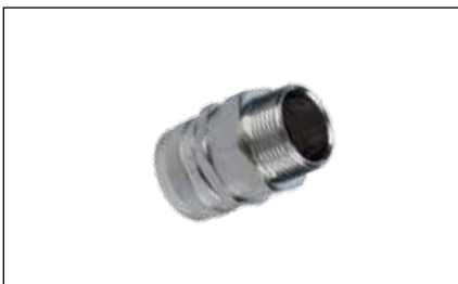
SG-M25... Nickle plated brass swivel gland M25, used with the M25-X-Ex e NP gland for termination of Thermon stainless steel conduit. Allows stainless steel conduit to freely rotate when gland is secured
