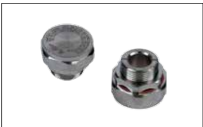
DPB-M25... Nickle plated Brass drain plug/Breather. Includes M25 lock nut. For use as a drainplug when installed in the bottom of Junction Box SS. Can also be utilized as a breather when installed in the top of an enclosure. For use in unclassified and potentially explosive atmospheres in accordance with the ATEX directive and IECEx Scheme. Ingress protection IP66.
