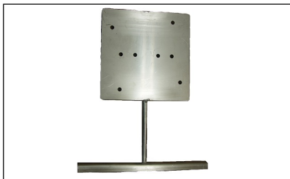
XP-1-150... predrilled 316 stainless steel mounting for mounting Thermon JB-SS-150 Junction Boxes, The bracket is easily secured to the pipe using 2 x B-10 attachment bands (Supplied). The XP-1-150 utilises a 110-mm standoff.
