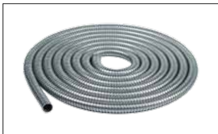
Flexible Conduit SS-25... Flexible conduit, 316 Stainless Steel for use with SG-M25. OD: 25mm, ID:21.1mm, IP40
