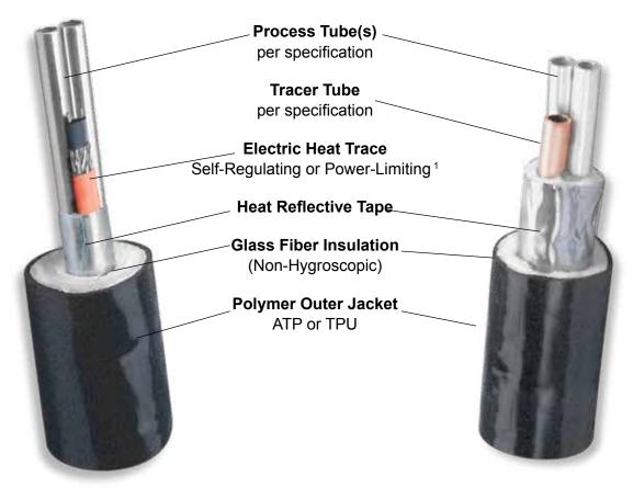
Standard TubeTrace Bundles are designed so the outer jacket will not exceed 60°C when the process tube is 204°C<sup>2</sup> and the ambient is 27°C, no wind.
