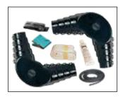
90° Large Elbow Transition Kit is designed to make a waterproof seal over TubeTrace elbow splices. FAK-2 [fits 32 mm-51 mm (1-1/4"-2") O.D. bundles] FAK-2L [fits 57 mm-89 mm (2-1/4"-3-1/2") O.D. bundles]
