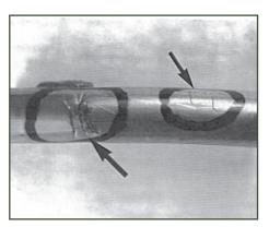
Chloride ion induced stress corrosion cracking (SCC). Failure initiated from the inside of the tube.
