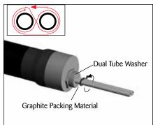
**29.** Slide a dual tube washer over the tubes to make contact with the fitting. Wrap graphite packing material around the tubing. See inset for details.
