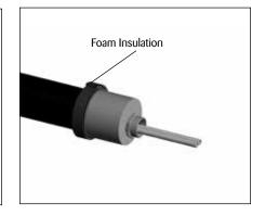
**26.** Wrap the foam insulation around the tubing bundle jacket.
