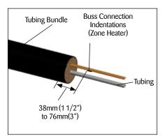
**1.** Remove outer jacket and insulation from the end of the tubing bundle. Strip back bundle insulation 38mm (1 1/2") to 76mm(3") <u>beyond buss connection</u> heat tracing.
