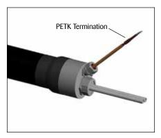
**18.** Terminate the heat trace with the appropriate PETK kit. Refer to the PETK Installation Instructions for details.
