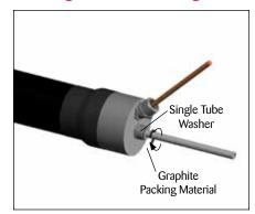
7. Slide a single tube washer over the tube to make contact with the fitting. Wrap graphite packing material four complete wraps around the tubing and press into the cavity on the tube fitting. Cut away excess graphite packing material.
