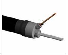
**17.** Tighten fitting nut to compress grommet against the heat tracer.
