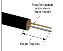
**2.** If buss connection indentation is less than 381mm (15") from end of the heat tracing, proceed stripping the bundle insulation to the next indentation.
