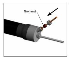
**10.** Slide the single or dual grommet and heat trace fitting nut over the heat tracer(s).
