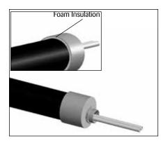
**27.** Slide foam insulation into the area between the tubing bundle end seal and the tubing bundle jacket routing the tubes through their designated openings. Be sure the tubing bundle end seal lid touches the end of the bundle.
