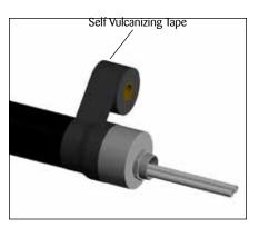
**28.** Wrap the self vulcanizing tape around the bundle jacket. Continue wrapping the tape around the bundle and end cap making sure to overlap each wrap by 50%.
