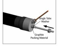
**8.** Slide the second single tube washer and the fitting nut over the tube.
