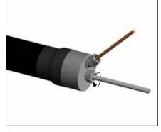
**9.** Tighten nut, compressing the washers and packing material into the fitting cavity.
