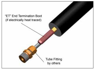
Deburr end of tubing and make necessary field installation connections. If tubing is electrically heat traced, make-up end termination and/or power connection per instructions included with the appropriate termination kit. (order separate from the FAK-7)
