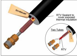
Liberally apply RTV sealant to tubing bundle insulation. For multi-tubes, apply RTV between the tubes.
