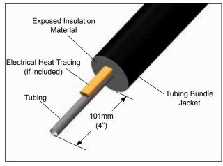
1. Strip back insulation approximately 101mm (4") from tubing bundle end
