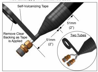
While removing the clear backing from tape, wrap end of tubing bundle with self-vulcanizing tape. Start a minimum of 51mm (2") above the cut on the outer jacket and continue a minimum of 51mm (2") along the bare tubing. Overlap the tape at least 50%. If electrically heat traced, it is recommended that the end termination be sealed and placed inside the insulation or at the connection, to assure no moisture enters the bundle insulation.
