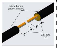
Remove outer jacket and insulation from tubing bundle approximately 127 mm (5") from end of the tubing bundle. Where required ensure sufficient heat trace is available for electrical splice. See instructions included with heat trace kit (purchased separately).
