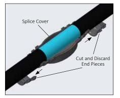
**6.** Cut top and bottom splice cover ends to match outside diameter of tubing bundle.
