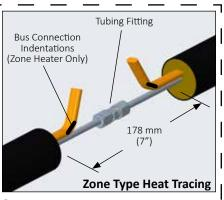
2a. If bus connection indentation is less than 38 mm (1.5") from end of the heat tracing, proceed stripping the bundle insulation to the next indentation.
