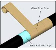
**4.** Wrap tube and heat trace with 1 pass of reflective tape (25% overlap), then wrap with 3 passes of glass fiber tape (50% overlap), or until fiber tape is equal to original bundle insulation thickness.
