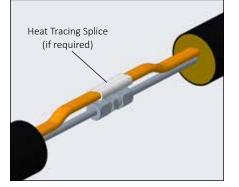
**3.** If bundle includes electric heat trace, make-up splice per instruction included with heat trace kit. This should be accomplished after fittings are leak tested.
