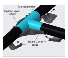
Cut top and bottom splice cover ends to match outside diameter of tubing bundle.
