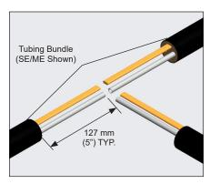
1. Remove outer jacket and insulation from tubing bundle approximately 127 mm (5") from end of the tubing bundle. Where required ensure sufficient heat trace is available for electrical splice. See instructions included with heat trace kit (purchased separately).
