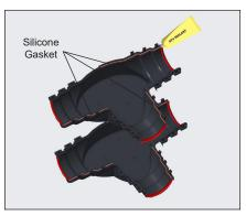
Install silicone gasket, cutting off excess. Apply RTV sealant to both halves.
