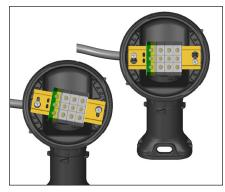
17. Install terminal block and complete system wiring. Terminal set screws shall be tightened to a torque value of 1.4 Nm (12.4 lb-in). See below for wiring details.
