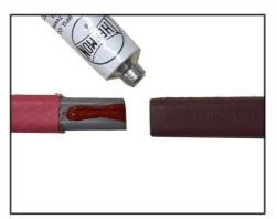
Apply a generous amount of RTV sealant to the cable end and inside the ET-6 end cap.
