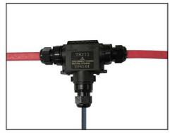
9. Close the Tee Box and screw the cable glands into the cover. Insert the cable gland gromment into the gland. Now tighten the nut on the gland. Do this for the other two glands. Do not over tighten the glands. This completes the HSX Power-2 connection.
