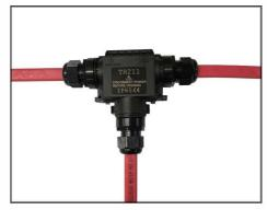
7c. Close the Tee box and screw the cable gland into the cover. Insert the HSX cable gland gromment into the gland. Now tighten the nut on the gland. Do this for the other two cables. Do not over tighten the glands. This completes the Tee connection.
