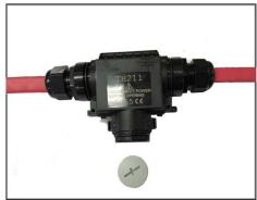
**8c.** Close the Tee box and screw the cable gland into the cover. Insert the HSX cable gland gromment into the gland. Now tighten the nut on the gland. Do this for the other cable. Do not over tighten the glands. Screw in the blanking cap into bottom section. This completes the In-line Splice connection.
