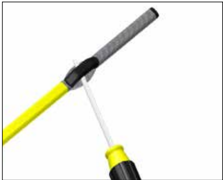
2. Separate braid strands at edge of overjacket and pull cable through opening in braid.
