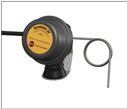
16. For ambient sensing applications, the mounting location should be representative of the coldest region, and the sensing element should not be exposed to direct sunlight or any additional heat source.
