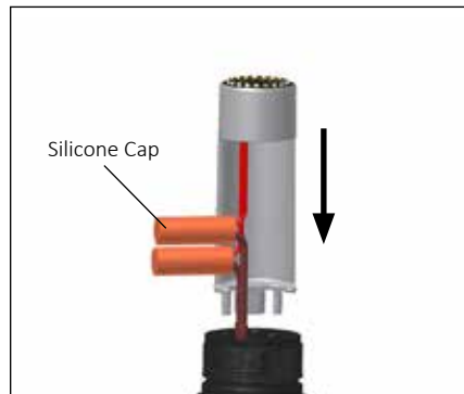
10. Slide silicone caps over crimp insulators. Install Light Module to Expediter.
