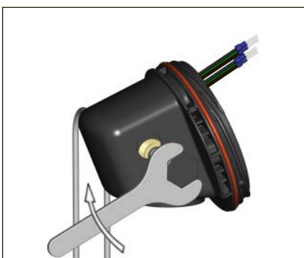
6. Install M20 blind plug in remaining M20 threaded entry (if necessary). Additional M20 blind plug (order M20-B-EXE) will be required if only installing one gland. Tighten existing blind plugs.
