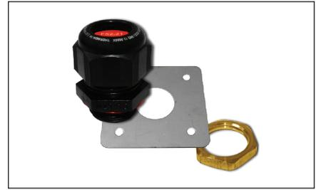
**Insulation Entry Kits (IEK)...** are used for inserting permanent circular and noncircular cables into the insulation. The kit protects and seals the cable while penetrating the insulation cladding.
