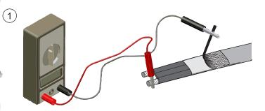
Connect the positive lead of the megger to the cable bus wires and the negative lead to the metallic braid.
