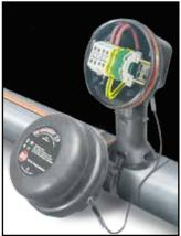
ZL . . . End-of-circuit light kit is designed to provide visual indication of an energized heating circuit. The kit may be utilized as an end termination or a power connection. Electrical connections are made in a terminal block utilizing nickel-plated copper terminals to ensure the electrical integrity of the connection over time.
