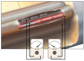
AC voltage will generate a current in the conductor which returns through the inside surface of the heat tube. There is virtually no measurable voltage on the outer surface of the heat tube, allowing the piping system to be grounded.
