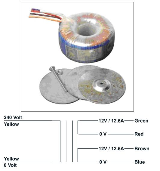
For 12 Volt operation: Join the **RED** and **BLUE** wires for one connection and the **GREEN** and **BROWN** wires for the other connection
