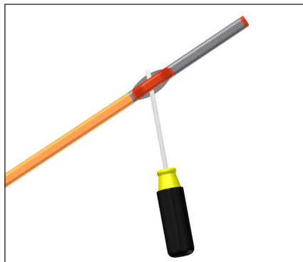
1b. Separate braid strands at edge of overjacket and pull cable through opening in braid.
