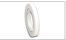
FT-1L fixing tape is used for attaching the heat trace to piping every 30 cm (12") or as required by code or specification. FT-1L may also by used for attaching pipe mounted expediters in circuit fabrication and splice kits. Tape is 13 mm (1/2") wide x 33 m (108') long.
