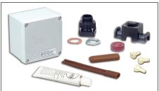
**PCA-COM** circuit fabrication kit is designed to fabricate an HSX 2100 circuit with one power connection boot and one end cap. Up to three HSX heat tracers can enter a PCA-COM kit when additional connection boots (TBX-3L) and end caps (ET-6) are used.
