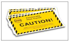
**CL** caution labels (vinyl-based peel and stick) should be installed on the thermal insulation weather barrier. In accordance with the NEC, electrically heated pipelines and vessels are to be clearly identified "at frequent intervals along the pipeline or vessel." Caution labels should be placed at 3-6 m (10'-20') intervals or as required by code or specification.
