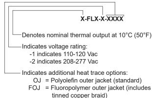
**Example** From the information obtained in Steps 1, 2 and 3, suppose an 8-FLX-1 heat trace will be required for a project. Since the application will have exposure to sea air, a standard polyolefin outer jacket is desired. The proper FLX for this application is: 8-FLX-1-OJ.
