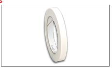
FT-1L fixing tape is used for attaching the heat trace to piping every 30 cm (12") or as required by code or specification. FT-1L may also by used for attaching pipe mounted expediters in circuit fabrication and splice kits. Tape is 13 mm (1/2") wide x 33 m (108') long. Max. Exposure Temp......93°C (200°F)
