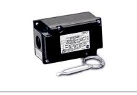
**N4X-40...**line-sensing thermostat is snapacting "open-on-rise" and preset at 5°C (40°F). Thermostat is rated for 125/250/480 Vac with a switch rating of 22 A and is housed in a NEMA 4X polycarbonate enclosure that is predrilled for connection to 3/4" conduit fitting. Thermostat has tinned copper bulb and capillary.
