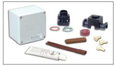
PCA-COM circuit fabrication kit is designed to fabricate an FLX circuit with one power connection boot and one end cap. Up to three FLX heat tracers can enter a PCA-COM kit when additional connection boots (TBX-3L) and end caps (ET-6) are used.
