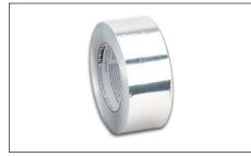
**AL-20L...**aluminum tape for securing cable on non-metallic pipe. Allow one foot of tape for each foot of heating cable. Tape is 51 mm (2") wide x 46 m (150') long.
