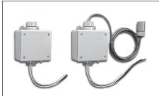
STC-DS-2B...stand-alone snow and ice sensor/controller is designed to operate on either 120 Vac or 208-240 Vac control power, includes a single 30 A normally open load contact rated to 277 Vac, and provides an adjustable temperature set point with manual on/off, automatic and standby switching functions.
