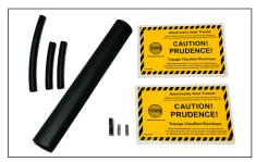
**HS-PBSK...**heat shrink in-line splice kit designed to join two RGS self-regulating heating cables together. The kit includes a heat shrink sleeve, two silicone sleeves, two butt connectors, and a caution label.
