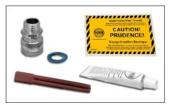
**18-SXG-KIT...**power connection kit is designed to fabricate an RGS circuit with one power connection boot and one gland fitting. The kit includes a cable transition fitting with watertight grommet and RTV adhesive. Power connection must be made in a suitable junction box such as the JB-K-L.
