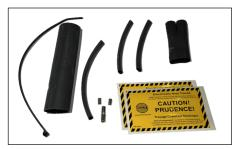
**HS-TBSK...**heat shrink T-splice kit designed to join three RGS self-regulating heating cables together. The kit includes one heat shrink tube, one heat shrink tee, two silicone tubes, two parallel connectors, one butt connector, one tie wrap, and a caution label.
