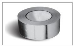
**AL-20L...**aluminum tape for securing cable in the bottom of a gutter. Tape is designed to hold cable in place and prevent movement during heavy rains. Allow one foot of tape for each foot of heating cable. Tape is 2" (51 mm) wide x 150' (46 m) long.
