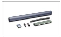
KSR-SK-DB...cable splice kit is designed to fabricate an in-line splice between two pieces of overjacketed cable. The kit allows for field fabrication of heating cable should the cable become damaged during installation. Easy-to-use kit includes splice lugs, self-vulcanizing tape and heat shrink tubing.
