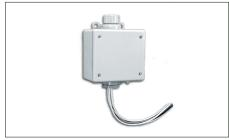
STC-DS-2B...stand-alone snow and ice sensor/controller is designed to operate on either 120 Vac or 208/240 Vac control power, includes a single 20 Amp normally open load contact rated to 277V, and provides an adjustable temperature set point with manual on/off, automatic and standby switching functions.
