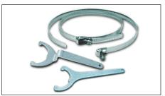
B-4, B-10, B-21 stainless steel attachment bands for securing Thermon JB-K nonmetallic kits and XP-1-140x140 mounting brackets to pipes. For pipes up to 100 mm, 250 mm and 530 mm diameters, respectively.
