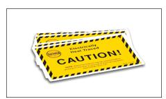
**CL** caution labels (vinyl-based peel and stick) should be installed on the thermal insulation weather barrier. In accordance with the NEC, electrically heated pipelines and vessels are to be clearly identified "at frequent intervals along the pipeline or vessel." Caution labels should be placed at 3-6 m (10'-20') intervals or as required by code or specification.
