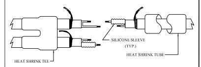
5. Slide heat shrink tee and heat shrink tube over cables. Slide short silicone sleeves over bus wires as shown.
