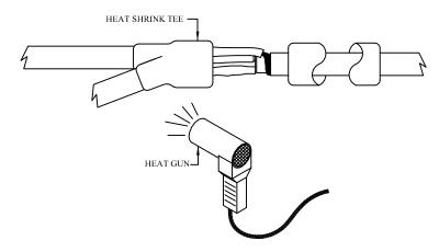
8. Slide heat shrink tee in place and use 700 Watt heat gun to heat shrink until encapsulant flows out each end of fitting.
