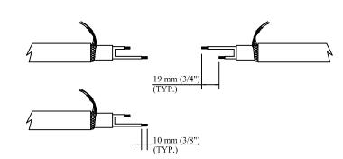
4. Remove 19 mm (3/4") of one bus wire from each cable, staggering bus wires as shown, so that the completed splices will not overlap. Strip 10 mm (3/8") of matrix material from end of all six bus wires.
