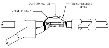
7. Slide long silicone sleeve over one braid wire as shown. Crimp metallic braid together using butt connector. Use T&B Cat. No. WT115A crimping tool (or equivalent T&B Cat. No.) on butt connector. Slide silicone sleeve over completed connection. Make sure that metallic braid does not touch black semi-conductive matrix.
