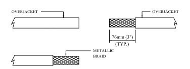
1. Remove 76 mm (3") of overjacket from end of each cable taking care not to cut metallic braid.
