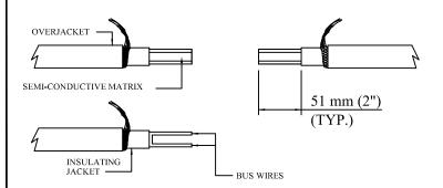
3. Remove 51 mm (2") of insulation from the end of each cable exposing the black semi-conductive matrix. Remove matrix material between bus wires of each cable. Leave black matrix material covering bus wires.
