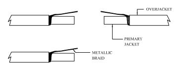
2. Twist metallic braid to form a pigtail. Fold braid back out of the way.
