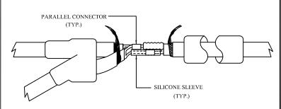
6. Crimp parallel connectors to make electrical tee splice connection. Use T&B Cat. No. WT111M crimping tool (or equivalent T&B Cat. No.) on parallel connectors. Slide silicone sleeve over each parallel connector.
