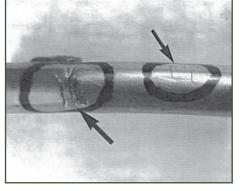
Chloride ion induced stress corrosion cracking (SCC). Failure initiated from the inside of the tube.
