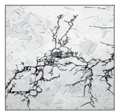
Photograph showing the typical "lightning bolt" cracking pattern associated with SCC.
