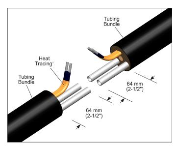
Strip back insulation approximately 2.5 in. (64 mm) from the end of the Pre-insulated Tube Bundle.
