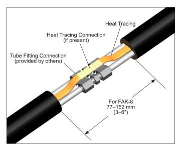
Make connections with appropriate fittings (provided by others). Test fittings for leaks before proceeding. If tubing bundle includes heat trace, make splice per kit instructions included with heat tracing.
