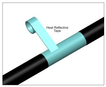
3. Wrap tube(s) with 1 pass of heat reflective tape (25% overlap). Then wrap with 3 passes of glass fiber tape (50% overlap). Complete with 1 additional pass of heat reflective tape.
