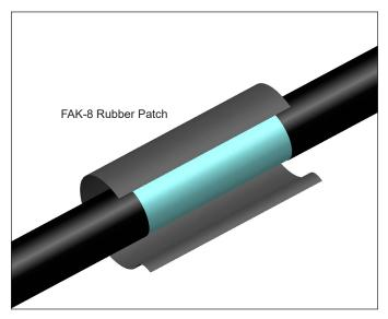
4. Cut a strip of FAK-8 patch long enough to wrap completely around the bundle and make a minimum overlap of 26 mm (1"). Wrap FAK-8 patch material over splice area overlapping outer bundle jacket to a minimum of 26 mm (1"). Press into place to form a water tight seal.
