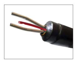
**10.** Apply heat to shrink sleeve, taking care to avoid pressing HPT heat trace up against tubing.
