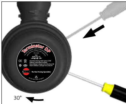
17. Install junction box lid and twist hand tight. Insert screwdriver into ratchet slot located on side of junction box base to tighten. Lid will rotate 30°.
