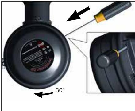
**16.** Install junction box lid and twist hand tight. Insert screwdriver into ratchet slot located on side of junction box base to tighten. Lid will rotate 30°.
