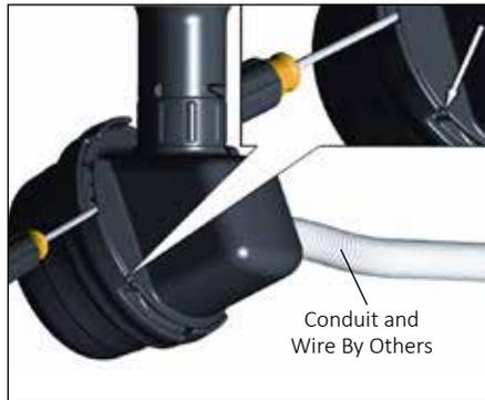
**17.** Lid latch mechanism fully engaged. To remove lid, repeat steps 15 and 16 but in opposite direction.
