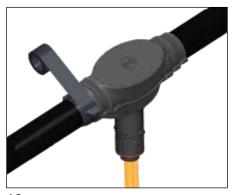
Apply self-vulcanizing tape around bundle jacket and work up over FAK ends.
