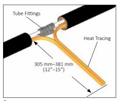
**3.** Make tube fitting connections with appropriate fittings (provided by others). Test fittings for leaks before proceeding.
