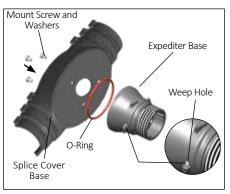
7. Mount expediter base with o-ring to the splice cover base using (3) M5 mounting screws and lock washers. Punch out weep hole.
