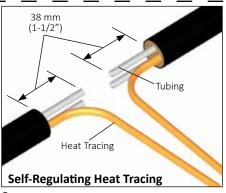
Trim tubing to within 38 mm (1-1/2") of the end of the insulation. If self regulating heat trace proceed to step 3. For Zone-type heat trace continue with identification of bus connection on step 2a.
