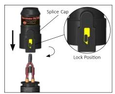
**15.** Mount splice cap to Terminator base, tighten securely. Make sure latch mechanism is in the locked position.
