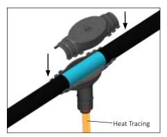
**9.** Assemble splice cover top, tubing bundle, and splice cover base together as shown. Snap together firmly. Inspect ends of tubing splice cover for snug fit. Apply additional RTV sealant where needed.
