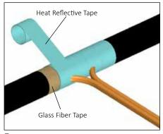
Complete with additional passes of heat reflective tape.
