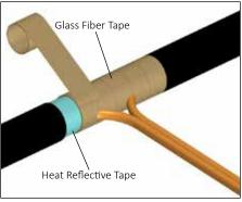
Wrap tubes and heat tracing with pass of heat reflective tape (25% overlap). Then wrap with 3 passes of glass fiber tape (50% overlap), or until fiber tape is equal to original bundle insulation thickness.
