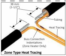
**2a.** Strip back bundle insulation 38 mm (1-1/2") to 76 mm (3") beyond bus connection indentation of each heat tracing. If bus connection indentation is less than 305 mm (12") to 381 mm (15") from end of the heat tracing, proceed stripping the bundle insulation to the next indentation. Trim tubes so the bus connection indentation on each meet.
