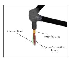
Terminate heat tracing with appropriate SCTK termination kit. Refer to SCTK installation instructions (purchased separately) for details not addressed here.
