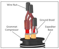
**12.** For splice connections: Connect bus wire using small wire nuts (for BSX, HTSX, KSX) or medium wires. (for RSX, VSX-HT, HPT, and FP). Connect braid wire using large wire nut. See wiring details for splice connections.
