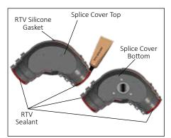
**8.** Install the Silicone Gasket (cut off excess). Apply RTV Sealant to both halves.
