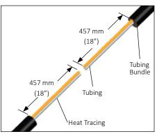
1. Remove outer jacket and insulation from tubing bundle approximately 457 mm (18") from end of the tubing bundle.
