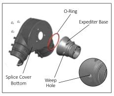
**7.** Mount expediter base with o-ring to splice cover bottom using (3) M5 mounting screws and lock washers. Punch out weep hole.
