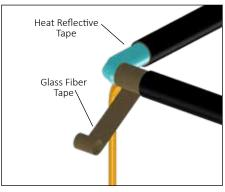
**4.** Wrap tube and heat trace with 1 pass of reflective tape (25% overlap), then wrap with 3 passes of glass fiber tape (50% overlap), or until fiber tape is equal to original bundle insulation thickness.
