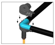
**9.** Assemble splice cover top, tubing bundle, and splice cover bottom together as shown Snap together firmly. Inspect ends of tubing splice cover for snug fit. Apply additional RTV sealant where needed.
