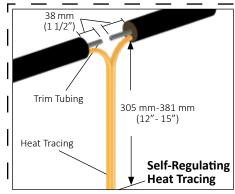
2. Trim tubing to within 38 mm (1-1/2") of the end of the insulation. If self regulating heat trace proceed to step 3. For Zone-type heat trace continue with identification of bus connection on step 2a.
