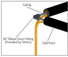
**3.** Make 90° elbow union connections (fitting provided by others). Test fitting for leaks before proceeding.
