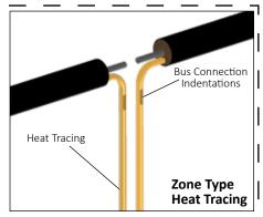
**2a.** Strip back bundle insulation 38 mm (1 1/2") to 76 mm (3") beyond bus connection indentation of each heat trace. If bus connection indentation is less than 305 mm (12")- 381 mm (15") from end of the heat tracing, proceed stripping the bundle insulation to the next indentation.
