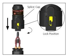
**14.** Mount splice cap to Terminator base, tighten securely. Make sure latch mechanism is in the locked position.
