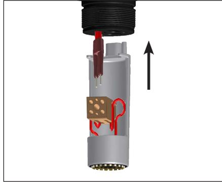
**18.** Connect the bus wires of the trace heater to the terminal block.
