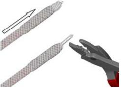
Slide the metallic braid over the end cap. Twist the ends of the metallic braid together and crimp with the lug.
