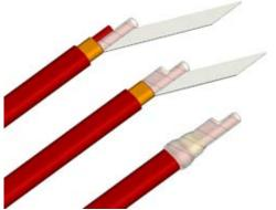
Tape bus wires individually and then together. Continue taping to cover overjacket.
