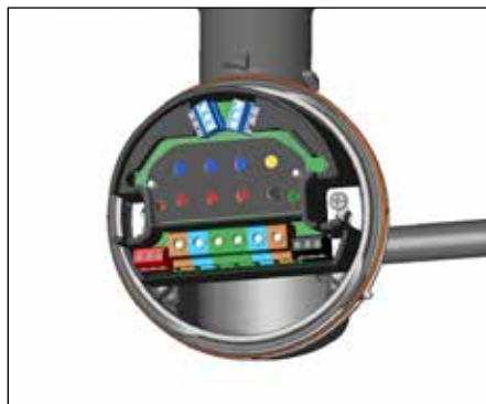
19. Install ECM electronic control module and complete system wiring. Terminal set screws shall be tightened to a torque value of 1,4 Nm (12,4 lb-in). See wiring details. Set ECM modules electronic control and/or control limiter at desired setpoints.
