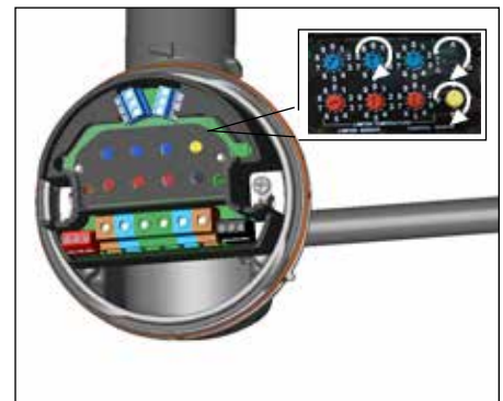
20. Use the rotary switches for settling Control and Limit Temperature, (Celsius or Fahrenheit) and Auto or Manual reset (Control switches on Type "C", Limiter switches on Type "L" and both on Type "CL"). Refer to ECM user manual for further details.
