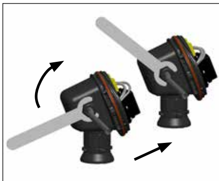
18. Remove M25 dust cap. Install M25 power gland (order separately) and M25 blind plug.
