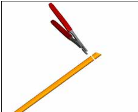
A1. Cut off end of cable.
