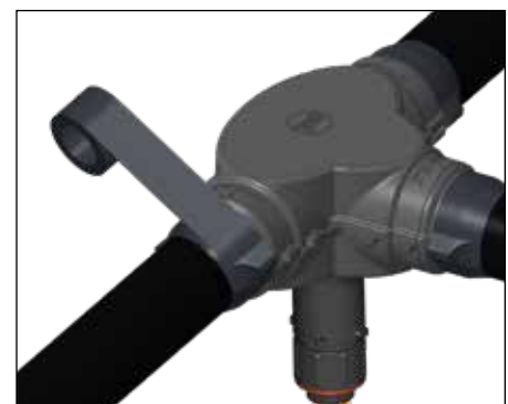
15. Apply self-vulcanizing tape around bundle jacket and work up over FAK ends.
