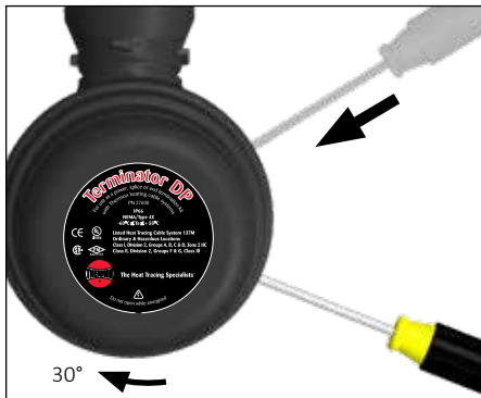
21. Install junction box lid and twist hand tight. Insert screwdriver into ratchet slot located on side of junction box base to tighten. Lid will rotate 30°.
