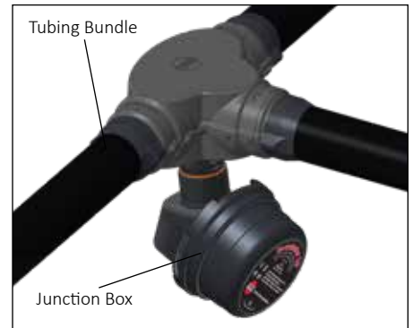
23. Completed Terminator DP/FAK-5LHT assembly for TubeTrace Type SE/ME Bundle.
