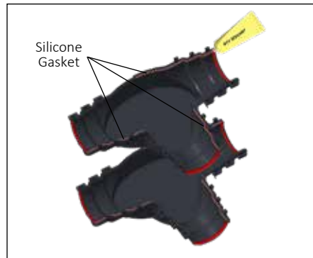
12. Install silicone gasket, cutting off excess. Apply RTV sealant to both halves.
